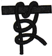
Round turn-and-two half hitches
